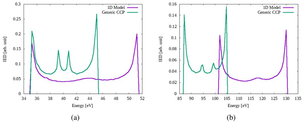
Figure 4: Fluid model IEDFs of (a) 6.64 Pa and (b) 2 Pa. In each figure, purple lines are at the wafer center of the 2D model, and green lines are the 1D model results.
