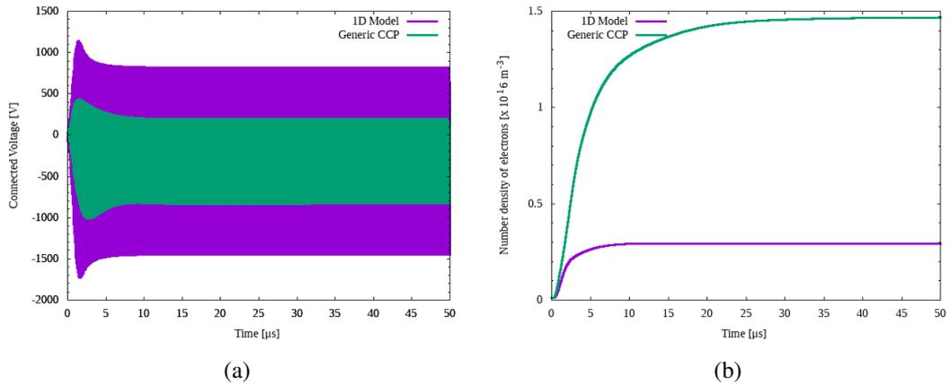
Figure 3: 2 Pa simulation results. (a) Connection voltage of the 2D model (green) and the 1D model (purple). (b) Transient of the number density of electron in the middle of the gap. The green line is the 2D model ( $r = 0$ ), and the purple line is the 1D model.
