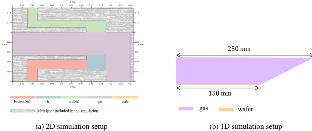
Figure 1: Model setup of simulations for (a) the 2D model and (b) the 1D model.
