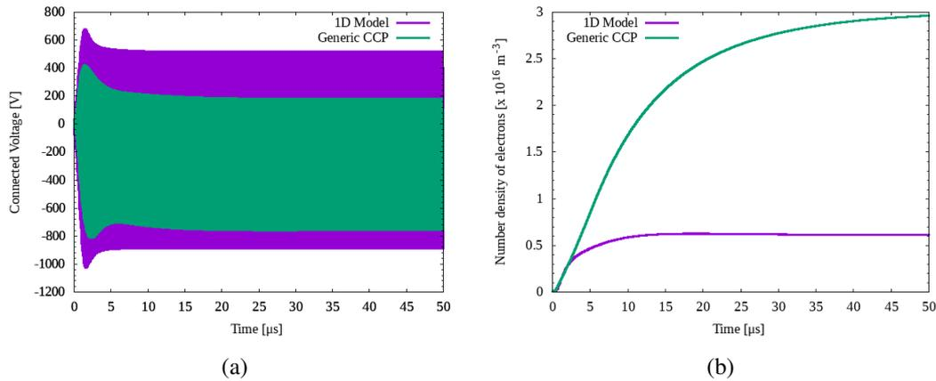
Figure 2: 6.64 Pa simulation results. (a) Connection voltage of the 2D model (green) and the 1D model (purple). (b) Transient of the number density of electron in the middle of the gap. The green line is the 2D model ( $r = 0$ ), and the purple line is the 1D model.
